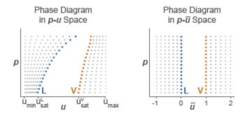
A pressure vector, of length N, and two normalized internal energy vectors, of lengths  $M_{\rm L}$  and  $M_{\rm V}$ , provide the  $(p, \bar{u})$  coordinates of the two grids. The pressure vector is common to both grids. The subcooled liquid grid is  $M_{\rm L}$ -by-N in size and the superheated vapor grid  $M_{\rm V}$ -by-N.
