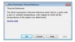
The Thermal Reference block has no parameters.
