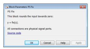
The PS Fix block has no parameters.
