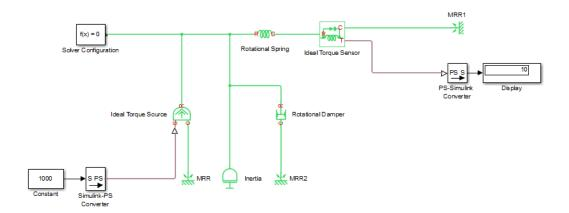
**Note** Currently, physical units are not propagated through the blocks in the Physical Signals library, such as PS Add, PS Gain, and so on. If your diagram contains a Physical Signals block after a Simulink-PS Converter block, the unit specification in the Simulink-PS Converter block does not propagate to the rest of the network.
