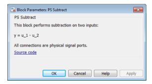
The PS Subtract block has no parameters.
