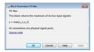
The PS Max block has no parameters.
