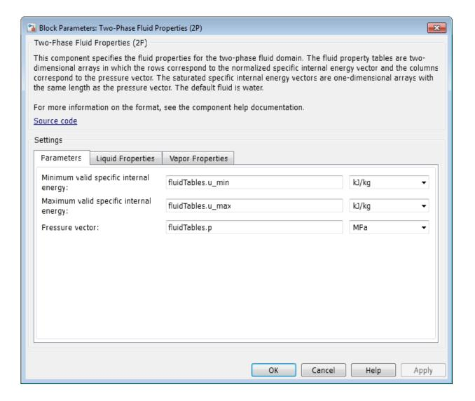
In the **Liquid Properties** tab, enter the field names from the fluidTables.liquid substructure as shown in the figure.
