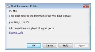
The PS Min block has no parameters.
